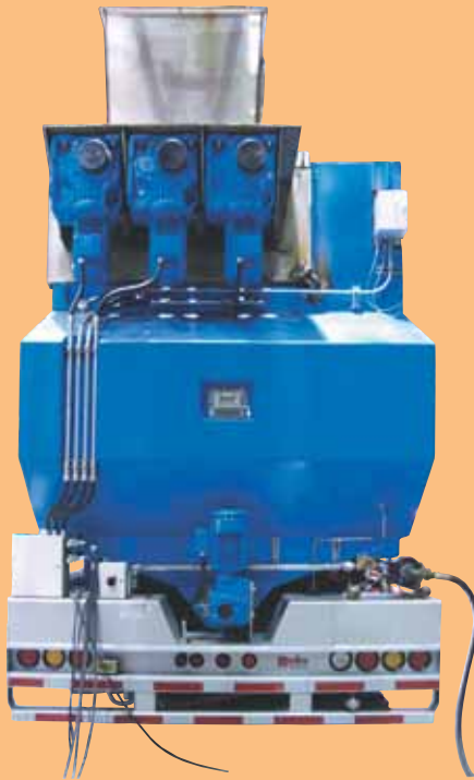
Large capacity thermal oxidizer on back of trailer with flame inspection window, and showing fuel supply (right) and feed system hook-ups (left).
