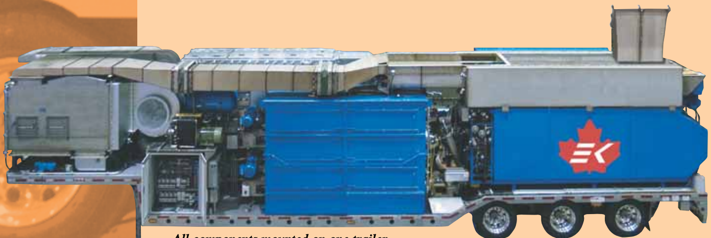
All components mounted on one trailer
