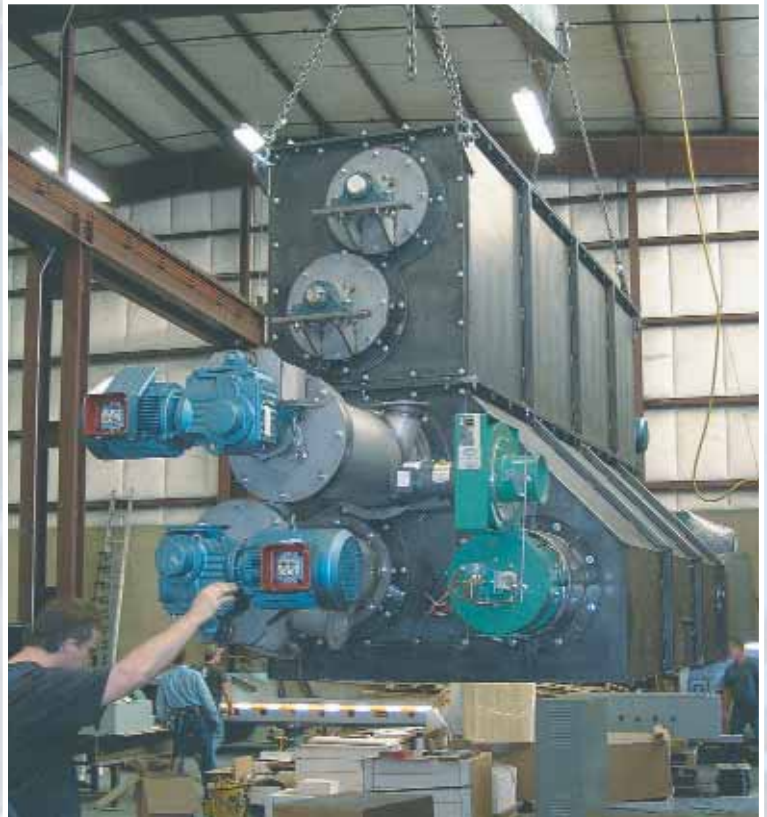
End view of the Enviro-Klean processor. Contaminated feed enters the top of the unit and cascades down through a series of chambers until the material is cleaned. On the lower left is a gas/oil processor burner.
