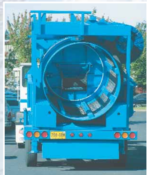
End view of feed trailer system showing the inside of the trommel screen with the opening into the dump hopper
