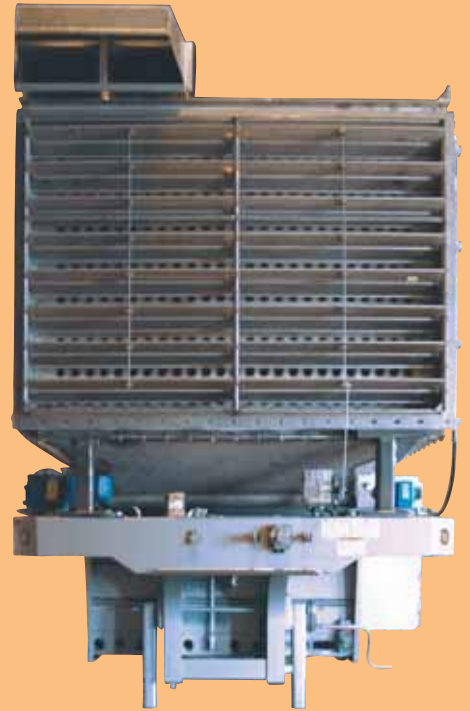
High efficiency 400-tube, air-to-air heat exchanger instantly reduces temperatures from 1000C to 200C (1800F to 400F) between the thermal oxidizer and baghouse.
